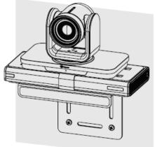
Example with the universal camera mounting shelf for wall mounting.
