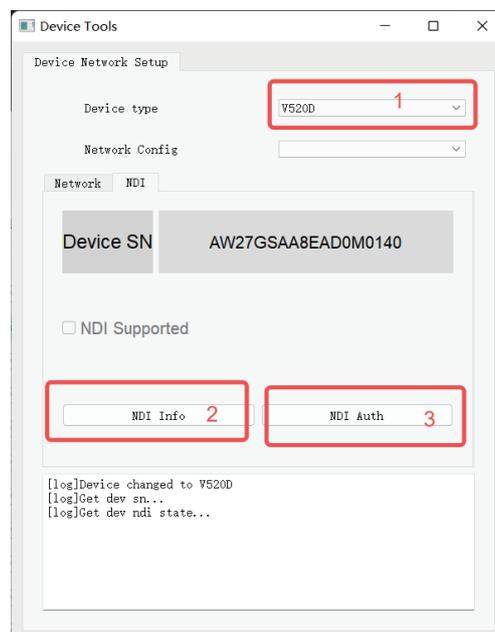
Make sure the camera and PC are on the same LAN and use the NDI tool to get the stream.
