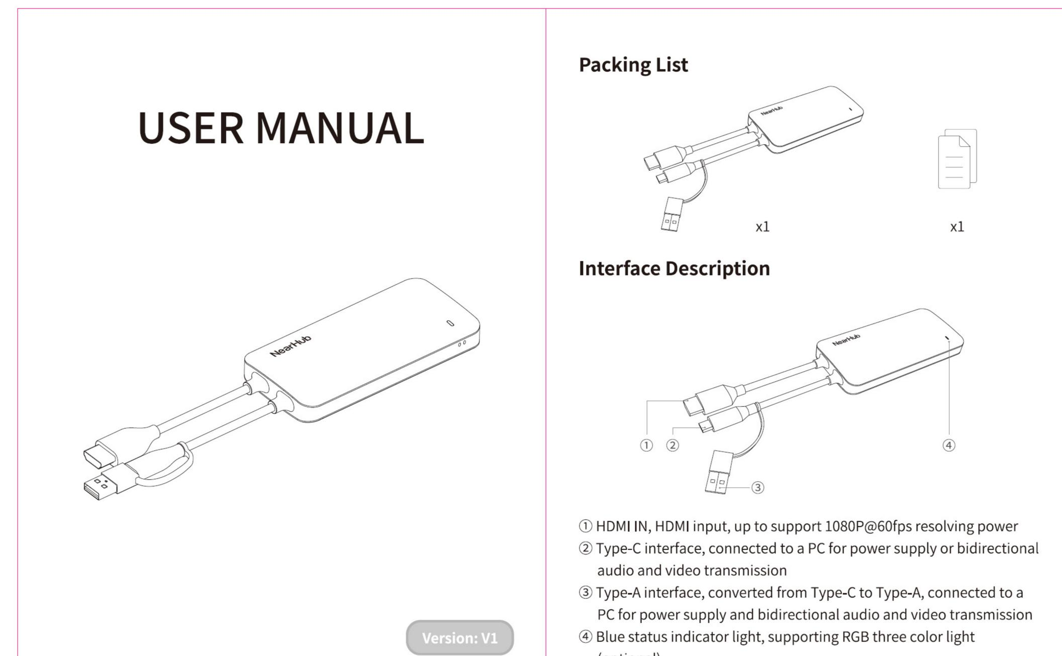
a. The Type-C port of the computer needs to support DP function, otherwise it will only be used for power supply or USB streaming of HDMI input transmission. b. HDMI and Type-C DP are either input, with HDMI having the highest priority. When HDMI is inserted, it is the HDMI input, and vice versa, it is the Type-C DP input. c. During HDMI transmission, Type-C power supply needs to be inserted simultaneously.
